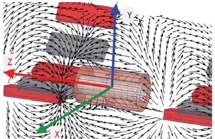
Figure 5. Flow map of the magnetic induction field in the axial plane  $y-z$ , related to a rotation of  $10^{\circ}$  of the magnets. It has been pointed out a bigger density of the flow lines in proximity of the  $x-y$  plane of the solenoid. The red magnets have the magnetic axis with the same sense and direction of  $z$ -axis while the gray magnets are opposite in sense.
