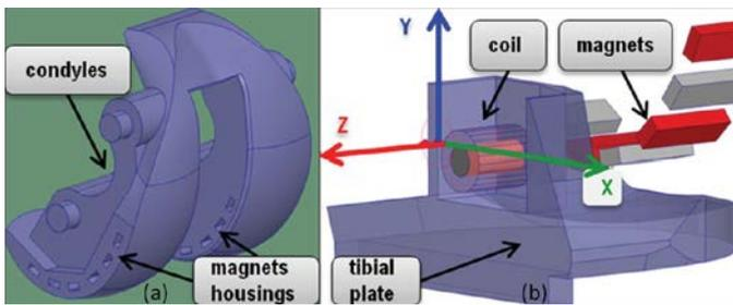
Figure 1. Femoral insert (condyles) of the knee prosthesis and a section, in the x-y plane, with the component of the electromagnetic generator.
