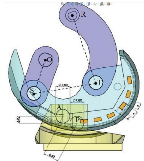
Figure 3. Motion system of the knee prosthesis.
