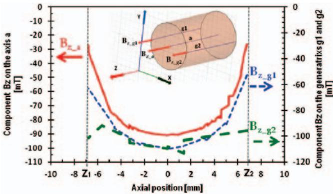
Figure 6. Function trend of z-component of the magnetic induction field on the coil A in the  $10^\circ$  configuration. The solenoid is positioned along z-axis between the coordinates  $z_1$  and  $z_2$ .
