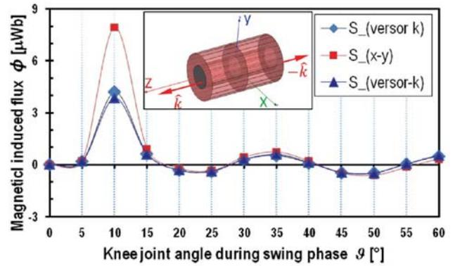
Figure 4. Function trend of magnetic flux, induced on three sections of the solenoid, indicated in Figure, in different angular positions of the magnets respect to coil A.
