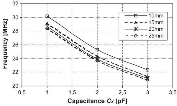
Fig. 11. Diagrams of  $f_a$  for different distances and different values of  $C_x$ .
