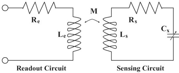
Fig. 1. Model that is commonly used to analyze telemetric systems.
