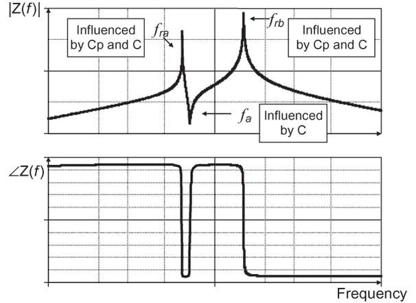
Fig. 4. Qualitative frequency response for typical parameters value of a telemetric system.
