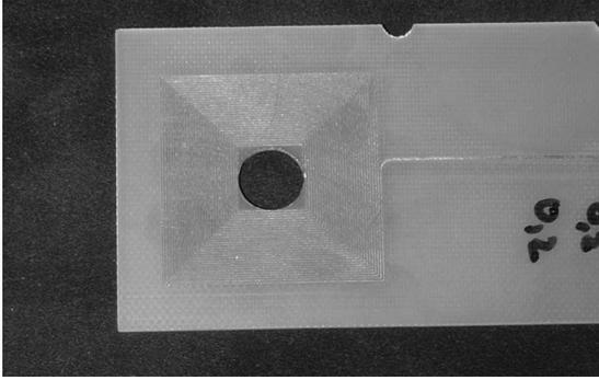
Fig. 5. Realized planar inductor.
