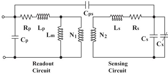
Fig. 2. Physical model of a system composed of two coupled planar inductances.
