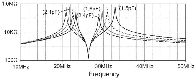
Fig. 8. Impedance module of the circuit of Fig. 3 with different values of  $C_p$ .
