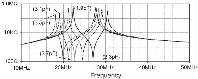
Fig. 7. Impedance module of the circuit of Fig. 3 with different values of  $C_c$ .
