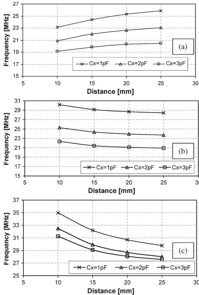
Fig. 12. Resonant frequencies (a)  $f_{r,a}$  and (c)  $f_{r,b}$  and (b) the frequency  $f_a$  for different values of sensing capacitance and different distances.
