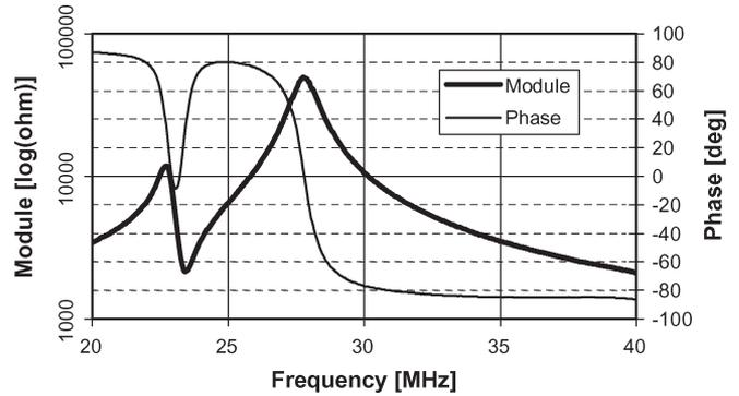
Fig. 10. Diagram of the impedance of the system measured on the readout with  $C_x = 2$  pF at 25 mm.
