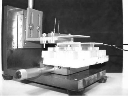
Fig. 6. Experimental system structure to obtain a measurable distance between the readout and sensing circuits.
