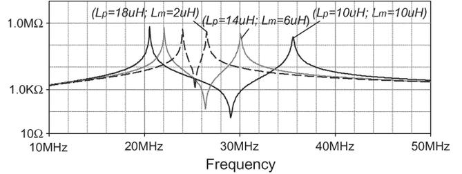
Fig. 9. Impedance module of the circuit of Fig. 3 with different values of  $L_m$ ,  $L_p$ , and  $L_s$ .
