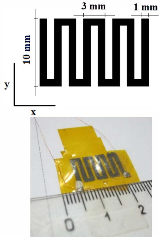
Fig. 1. Images of the realized strain gauge and dimensions.
