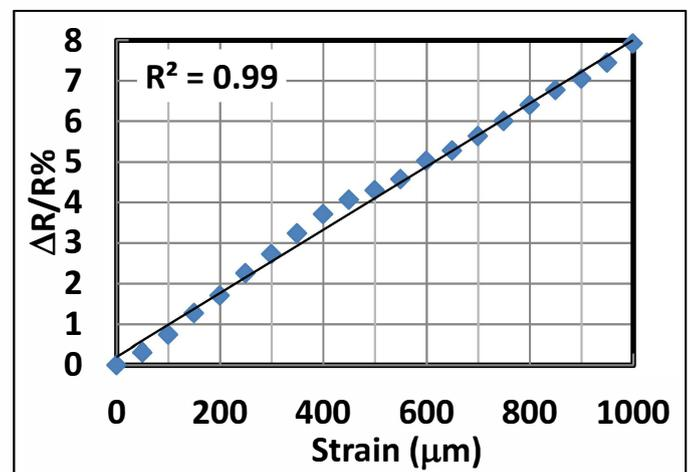
Fig. 6. Percentage change of the resistance vs. strain.
