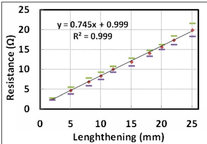
Fig. 3. Resistance values for different lengths of conductor.
