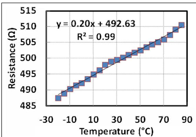
Fig. 4. Variation of the strain gage resistance vs. temperature.
