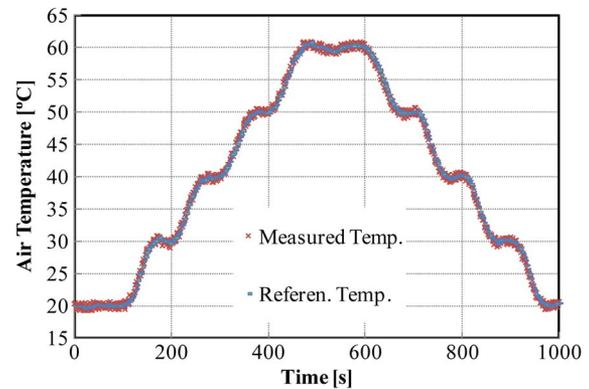
Fig. 9. Calculated values of air temperature, compared with the values obtained with the reference Pt100.
