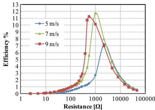
Fig. 6. Efficiency of the dc servomotor at different airflow velocities.
