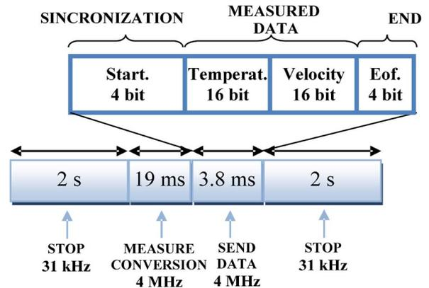
Fig. 3. Typical self-powered wireless sensor activities.
