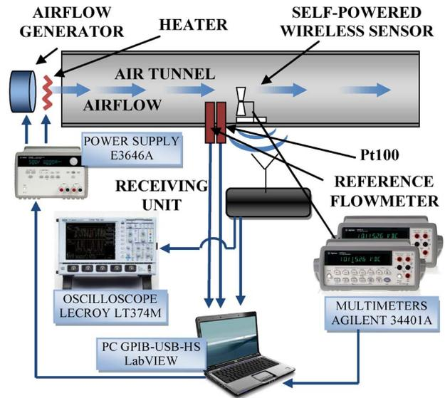
Fig. 4. Schematic diagram of the experimental system.
