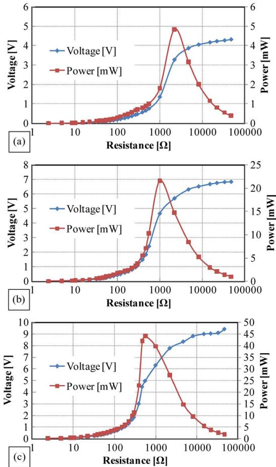
Fig. 5. Generated voltage and power by the dc servomotor at different airflow velocities. (a) 5 m/s. (b) 7 m/s. (c) 9 m/s.
