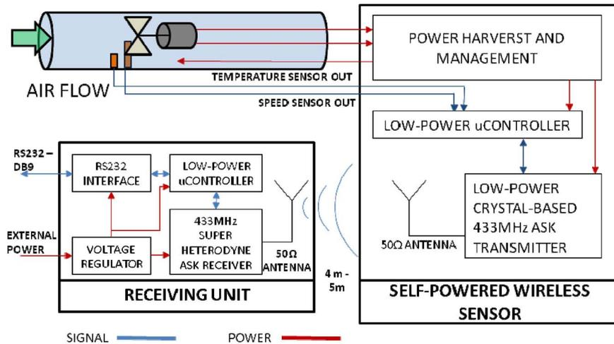
Fig. 2. Block diagram of the autonomous sensor and readout system.
