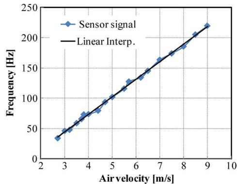
Fig. 8. Frequency values versus different airflow velocities.
