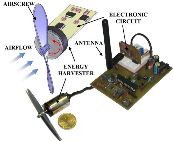
Fig. 1. Schematic diagram of the autonomous sensor.
