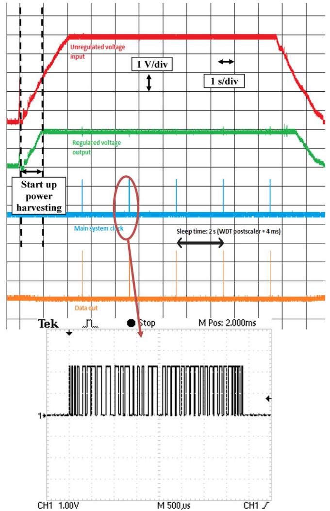
Fig. 7. Wake-up signals of the self-powered wireless sensor.
