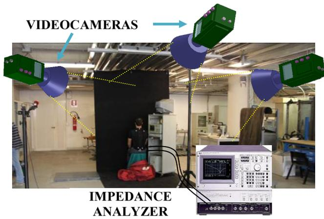
Fig. 4. Schematic diagram of the experimental system adopted for posture measurements.
