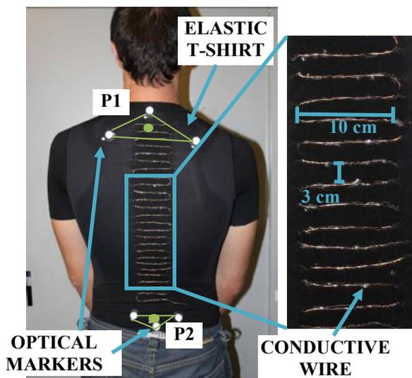
Fig. 2. Image of the inductive sensor realized over the T-Shirt.
