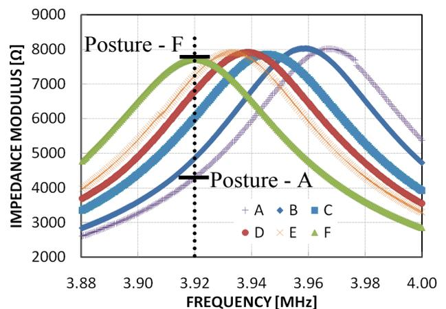
Fig. 7. Impedance measurement at different postures.
