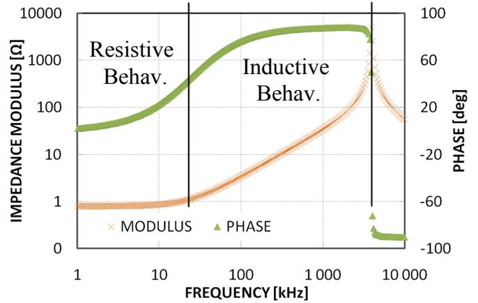
Fig. 6. Inductive sensor characterization.
