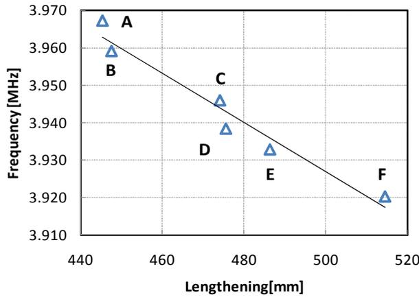
Fig. 8. Comparison between optical and resonant frequency measurements.
