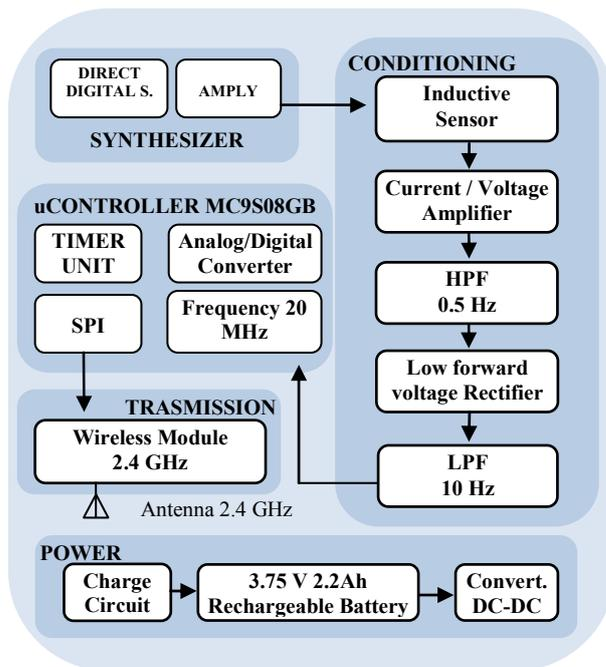
Fig. 3. Block diagram of the proposed conditioning electronics.
