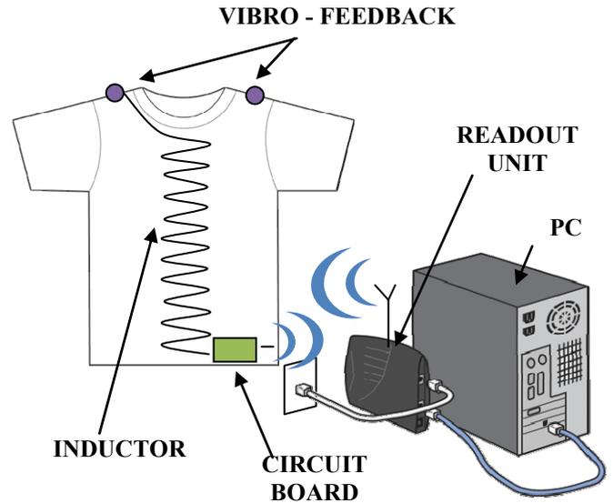
Fig. 1. Block diagram of the wearable system.
