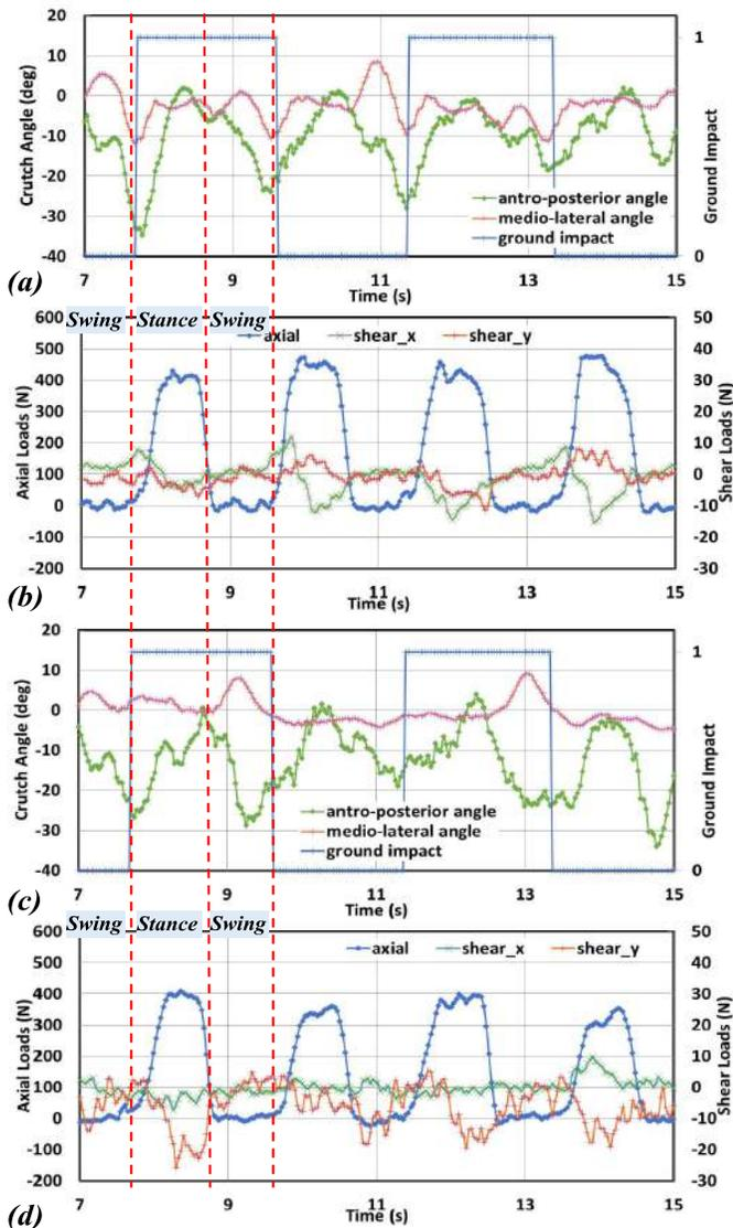
Fig. 10. Axial and shear loads and tilt angles monitored in real time during NWB tests of Subject1. (a) Left crutch angles. (b) Left crutch loads. (c) Right crutch angles. (d) Right crutch loads.
