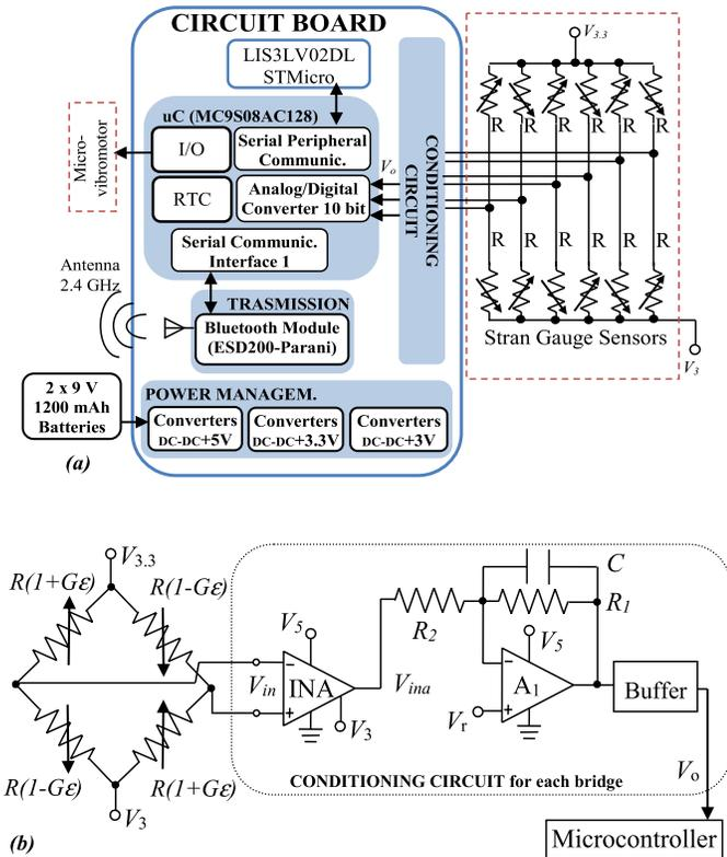
Fig. 3. (a) Block diagram of the circuit board for each wireless instrumented crutch. (b) Schematic of the conditioning circuit for each bridge.
