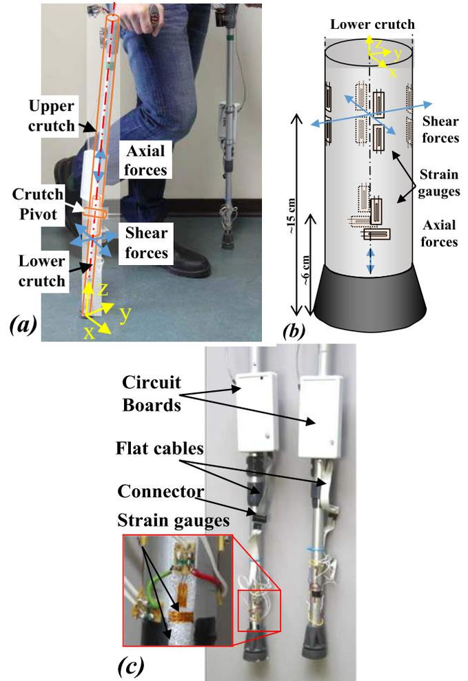
Fig. 2. (a) Crutch constitutional elements and forces. (b) Image of the strain-gauge positions. (c) View of mounting solution.
