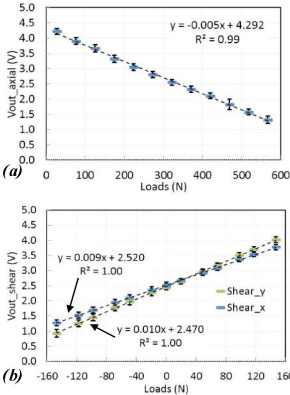
Fig. 7. (a) Axial force tests, conditioning circuit output voltages versus mechanically applied loads (mean and 3SD)—left crutch. (b) Shear force tests, conditioning circuit output voltages versus mechanically applied loads (mean and 3SD)—left crutch.
