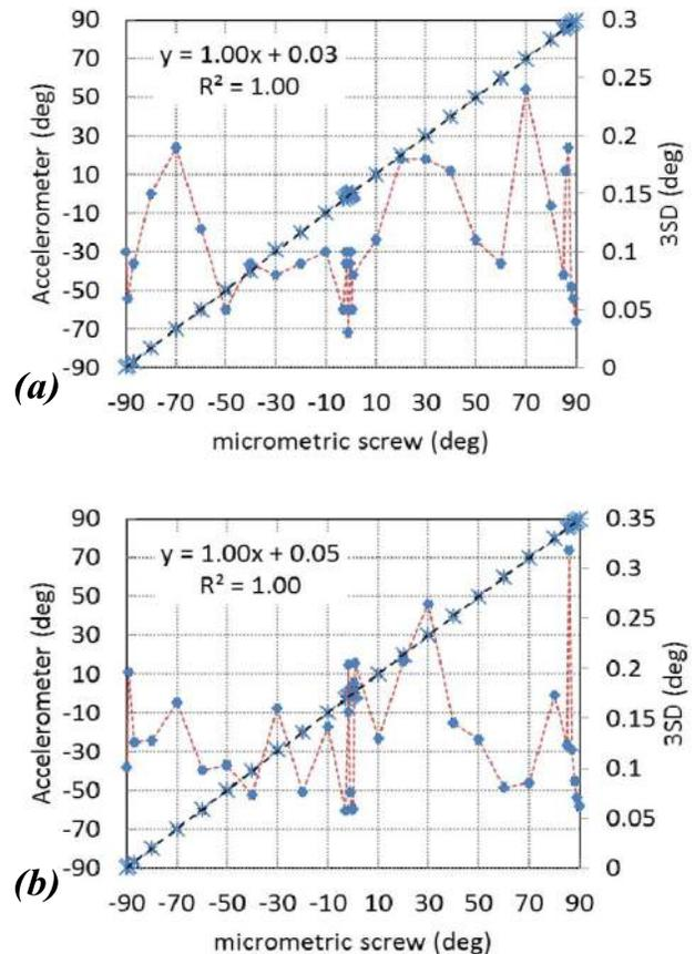
Fig. 6. Antro-posterior angle tests, mean (green dots), and standard deviation—3SD (blue squares) for the (a) left crutch and (b) right crutch.
