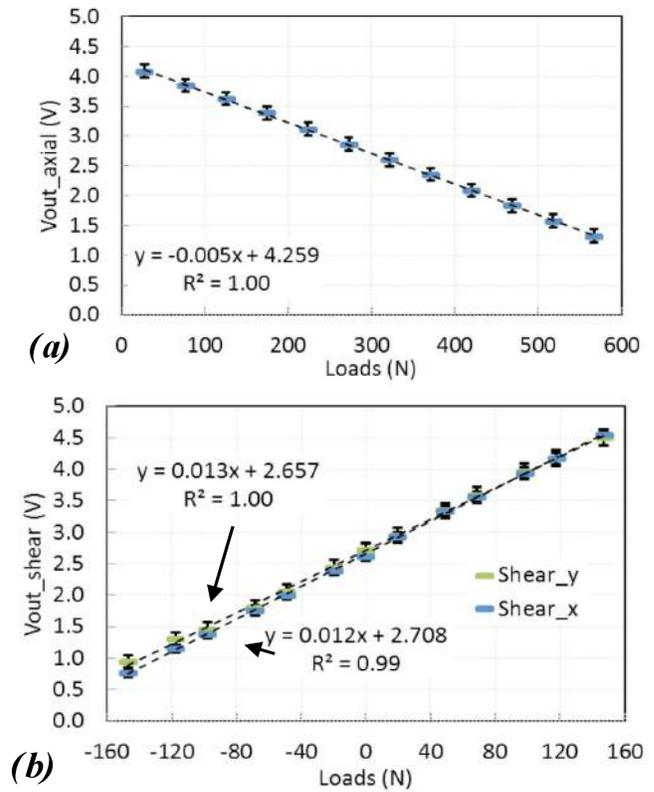
Fig. 8. (a) Axial force tests, conditioning circuit output voltages versus mechanically applied loads (mean and 3SD)—right crutch. (b) Shear force tests, conditioning circuit output voltages versus mechanically applied loads (mean and 3SD)—right crutch.
