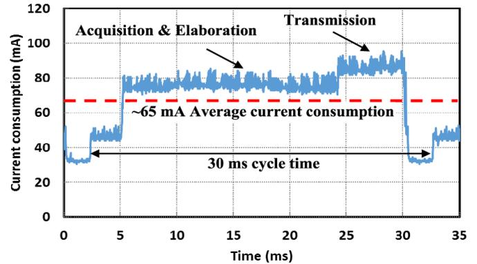
Fig. 9. Current consumption during one cycle.
