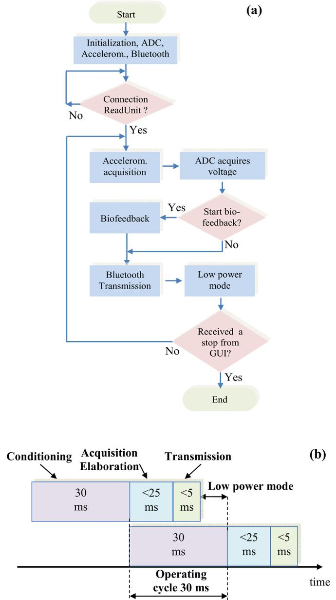
Fig. 4. (a) Schematic flowchart associated with the acquisition and transmission activities. (b) Schematic of an operation cycle.
