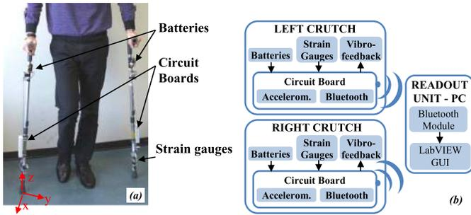
Fig. 1. (a) Picture of the wireless instrumented crutches. (b) Block diagram.
