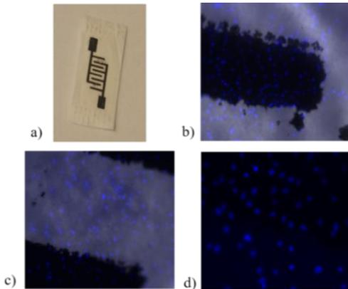
Fig. 2: a) Representative image of carbon on PCL sensor; b) Representative image of sensor with myoblasts stained with DAPI. The myoblasts appear adherent and evenly distributed both on PCL (c) and Carbon (d).
