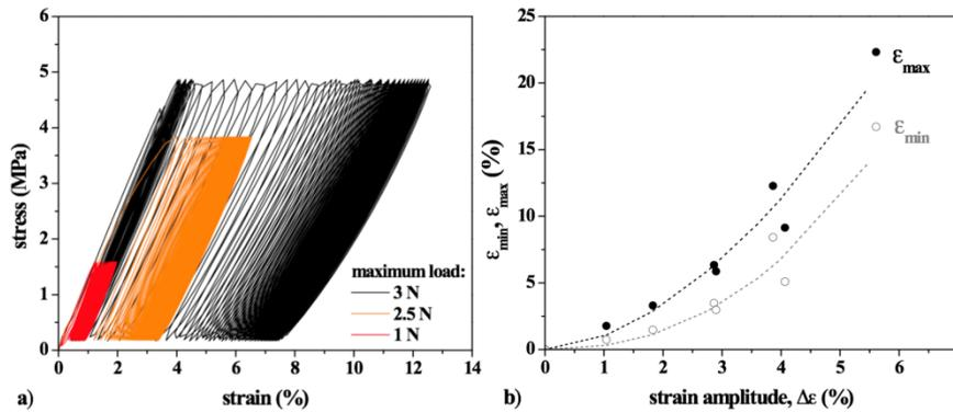
Fig. 1: a) Cyclic stress vs. strain curves for the crosslinked PCL scaffold subjected to various values of maximum load; b) Maximum and minimum strain values required to assure a given strain amplitude
