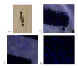
Fig. 2: a) Representative image of carbon on PCL sensor; b) Representative image of sensor with myoblasts stained with DAPI. The myoblasts appear adherent and evenly distributed both on PCL (c) and Carbon (d).
