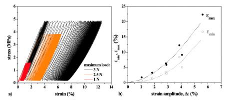
Fig. 1: a) Cyclic stress vs. strain curves for the crosslinked PCL scaffold subjected to various values of maximum load; b) Maximum and minimum strain values required to assure a given strain amplitude
