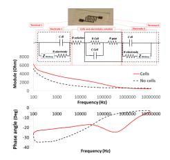
Fig. 3: Comparison between impedance module and phase angle with and without seeded cells and a schematic representation of the equivalent circuit model.
