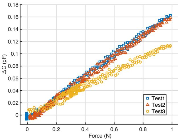
Fig. 7: Capacitance variation versus force. Test1 and Test2 are two different runs of the same test, maintaining the same force application position. Test3 is obtained moving the force application position from the spiral center
