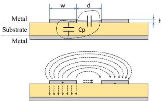
Fig. 2: Coplanar capacitor with ground plane,  $C_p$  is then parallel between the two intrinsic capacitances, increasing the direct capacitance value.
