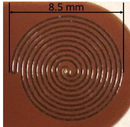
Fig. 5: (a) Section of the sensor. The widths are, copper 35  $\mu\text{m}$ , polyimide 25  $\mu\text{m}$ , PVS 2 mm and EVA 3 mm. The total sensor height equals to EVA's. (b) A picture of the polyimide machined layer, where, referring to Figs. 1 and 2, the dimensions are  $w = 0.203\text{ mm}$  and  $d = 0.1778\text{ mm}$ . The maximum diameter of the spiral is 8.5 mm.
