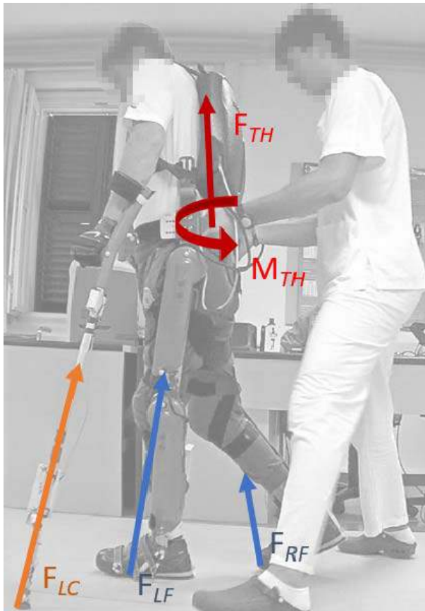
Fig. 1. A Rewalk™ user is supported by his physiotherapist during assisted gait training. The right leg is initiating the swing phase. External forces acting on patient-exoskeleton system are highlighted. F_{TH} and M_{TH} are, respectively the force and torque vectors applied by the therapist. F_{RF} and F_{LF} are the right and left foot ground reaction forces. F_{LC} is the left crutch ground reaction force. F_{RC} the right crutch is not displayed in the picture.
