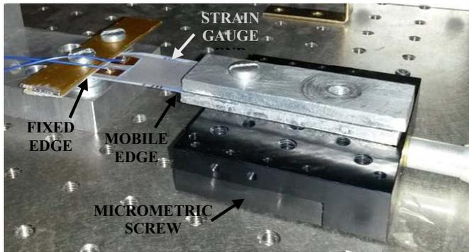
Fig. 4. Fixing apparatus adopted for strain tests.
