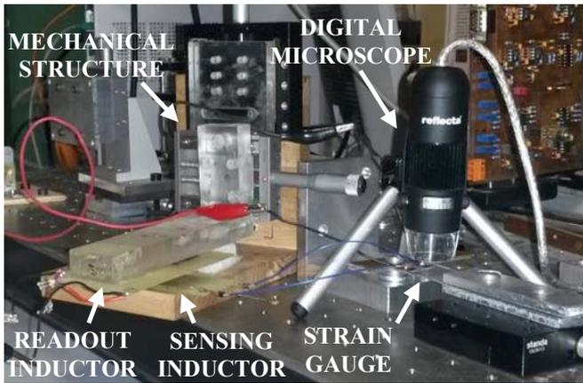
Fig. 8. View of the experimental apparatus for system frequency analysis.
