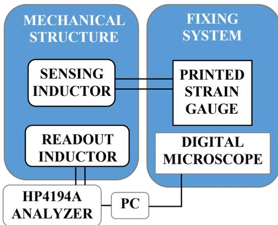
Fig. 9. Block scheme of the experimental apparatus.
