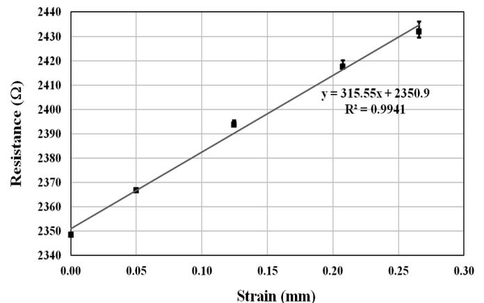
Fig. 7. Sensor characterization curve: resistance vs. applied strain.
