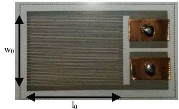
Fig. 3. Resistive strain gauge realized through inkjet printing technologies on a flexible substrate.
