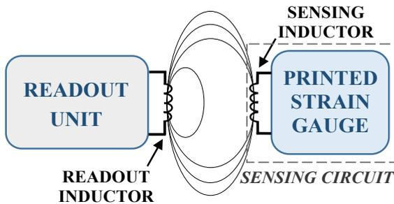
Fig. 1. Conceptual scheme of the proposed telemetric system.
