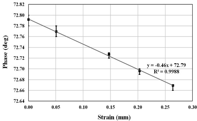
Fig. 11. Impedance phase minimum vs. applied strain. Distance between the inductors is fixed.
