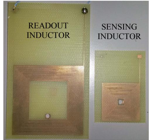
Fig. 2. Readout and sensing planar inductors.
