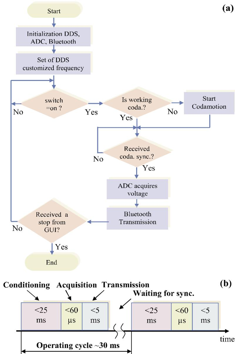
Fig. 6. (a) Schematic flowchart associated with the acquisition and transmission activities. (b) Schematic diagram of an operation cycle.
