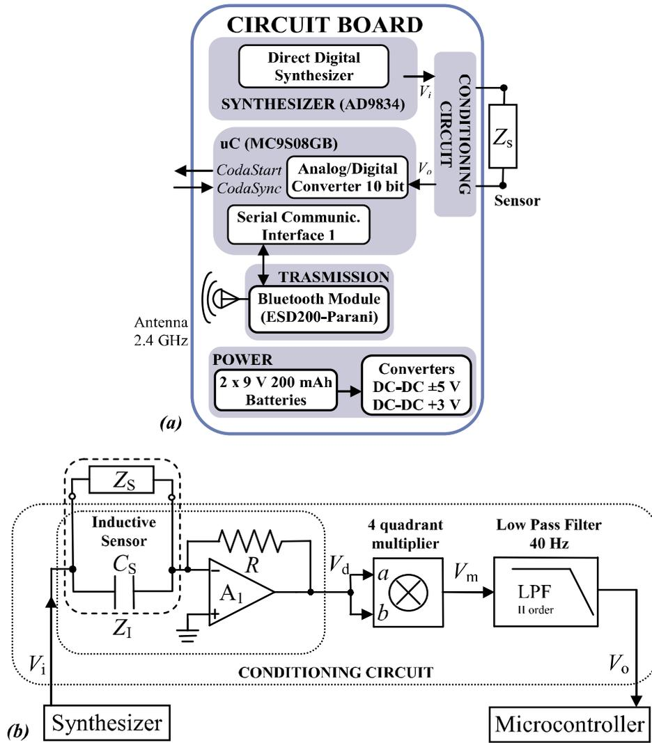
Fig. 5. (a) Block diagram of the circuit board. (b) Block diagram of the conditioning circuit.
