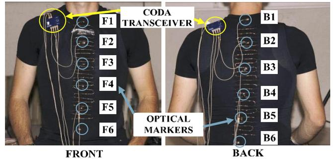
Fig. 8. Image of the inductive sensor realized over the T-shirt and the optical markers added for the comparison.
