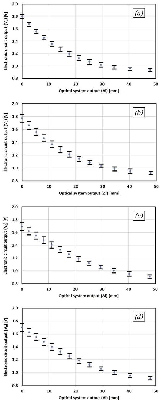
Fig. 10. Lengthening data obtained with the optical system versus the designed conditioning circuit (mean  $\pm$ 1 SD). (a) Subject 1. (b) Subject 2. (c) Subject 3. (d) Subject 4.
