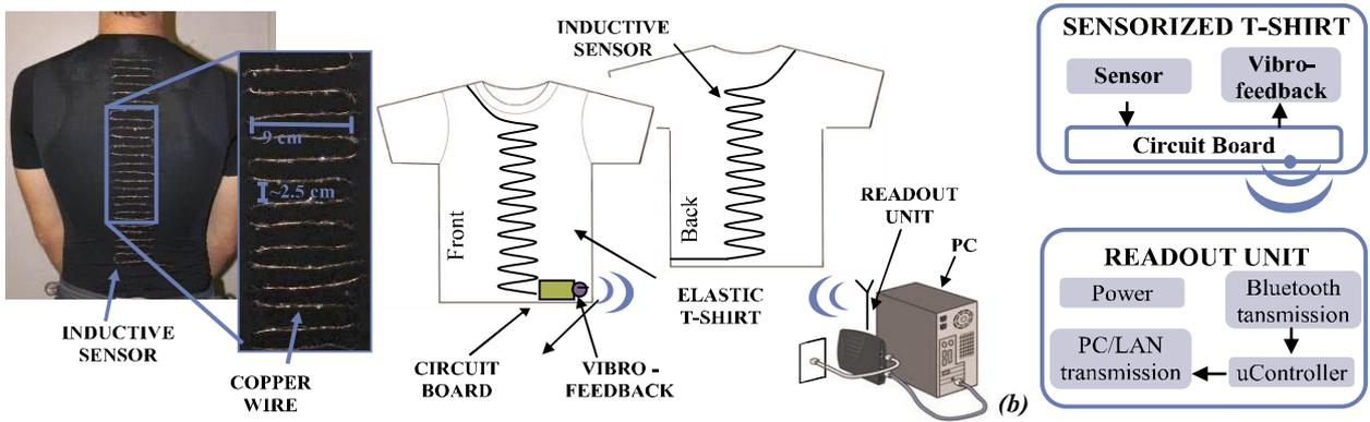
Fig. 2. (a) Posture monitoring system. (b) Block diagram.
