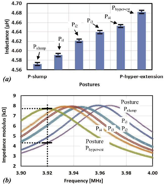
Fig. 4. (a) Sensor's inductance values at different postures (mean  $\pm 1$  SD) of one subject. (b) Impedance modulus measurement at different postures.
