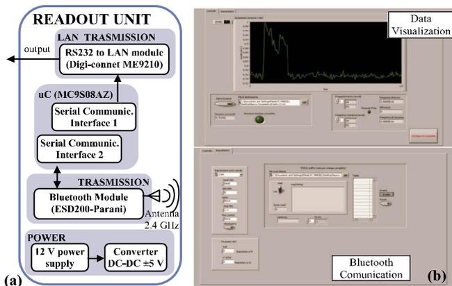
Fig. 7. (a) Block diagram of the read out unit. (b) Image of the realized GUI.
