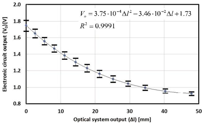
Fig. 11. Lengthening data obtained with the optical system versus the designed conditioning circuit (mean  $\pm 1$  SD) for all the subjects.
