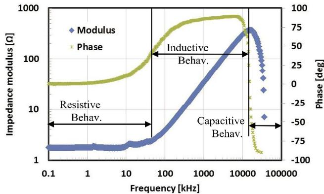
Fig. 3. Frequency behavior of the sensor.
