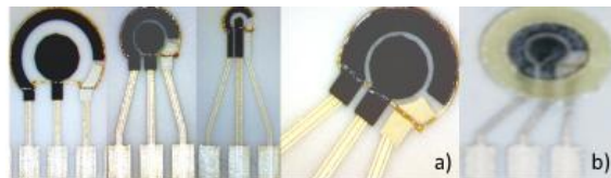
Fig. 2. a) Examples of the printed sensors on the alumina substrate, from left to right: 4 mm, 3 mm, 1 mm and 2 mm geometries; b) printed circuits with glued glass-fiber washers.
