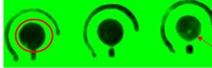
Fig. 3. Three alumina-substrate sensors covered by protein.
