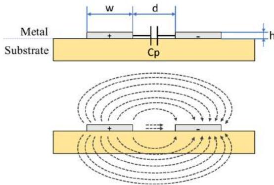
Fig. 1: Basic coplanar capacitor size and principle, where  $C_p$  is the intrinsic capacitance,  $w$  is the path width,  $d$  is the distance between them and  $h$  is the height of the metal layer.
