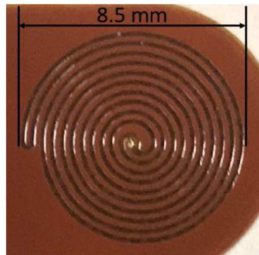
Fig. 5: (a) Section of the sensor. The widths are, copper 35  $\mu\text{m}$ , polyimide 25  $\mu\text{m}$ , PVS 2 mm and EVA 3 mm. The total sensor height equals to EVA's. (b) A picture of the polyimide machined layer, where, referring to Figs. 1 and 2, the dimensions are  $w = 0.203$  mm and  $d = 0.1778$  mm. The maximum diameter of the spiral is 8.5 mm.
