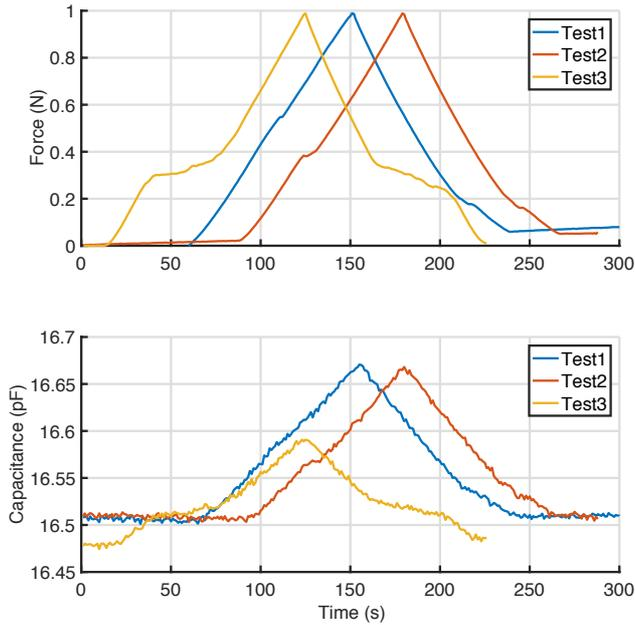
Fig. 6: Force values measured by the INSTRON load cell and the variation in the capacitance value of the sensor measured by the impedance analyzer.
