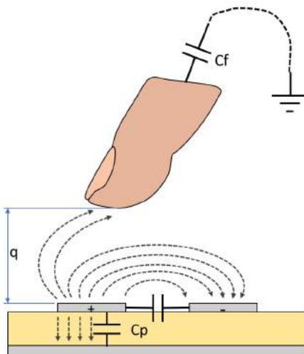
Fig. 3: When a finger (for example) approaches the coplanar capacitor, the capacitance value of the finger will change the total capacitance value of the sensor and it becomes  $C_{sens} = C_p + C_f$ . The capacitance variation is linked to the distance between the finger and the sensing element.
