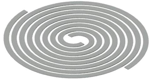
Fig. 4: Coplanar capacitor spiral design
