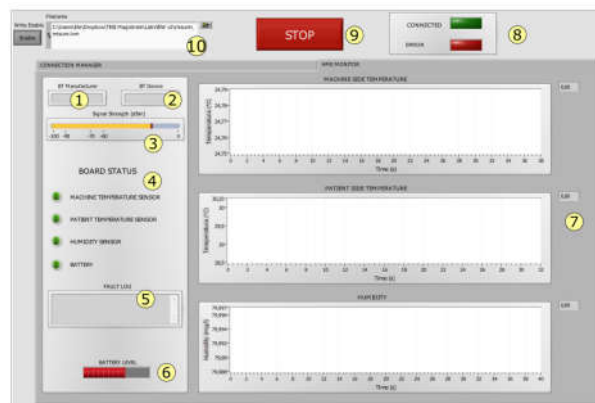
Fig. 4. LabVIEW measure monitor: (1) BT Manufacturer, (2) BT Device, (3) Signal Strength in dBm, (4) Board Status: green LEDs if OK, red LEDs if a fault is present, (5) Fault Log: a verbose description of the Fault Type and history, (6) Battery Level, (7) Measures: in this panel are represented, on a temporal chart and on a digital meter, absolute humidity and temperatures, (8) BLE connection status, (9) VI main stop, (10) Saving path of the measure file
