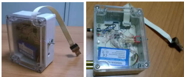
Fig. 3. Picture of the manufactured measuring section
