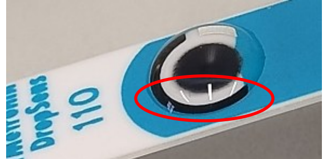
Fig. 6. Degradation of the ion-selective membrane after exposure to 1 M \text{NH}_4\text{OAc} .
