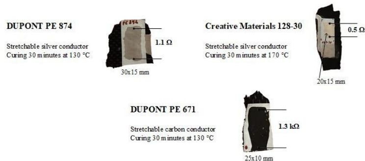
Fig. 3. Plate #1 realization: Conductive inks sample on polyurethane layer.
