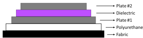
Fig. 2. Stack diagram of the soft capacitive force sensor.
