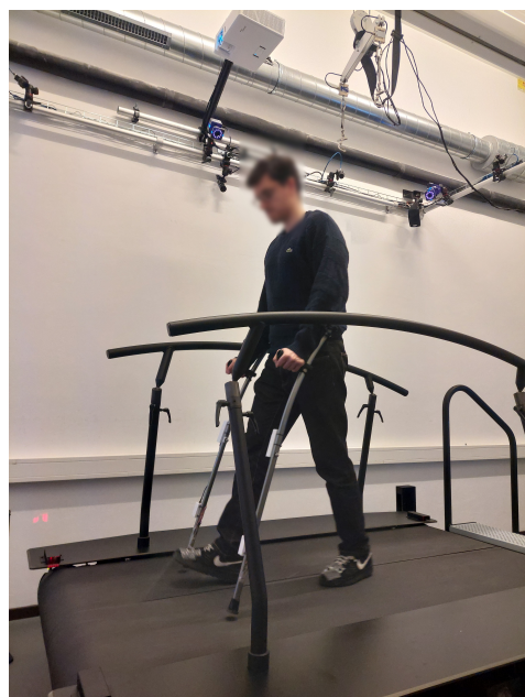
Figure 6. Representative example of a participant performing an assisted-gait trial on the instrumented dual-belt treadmill, surrounded by the Vicon infrared camera array.
